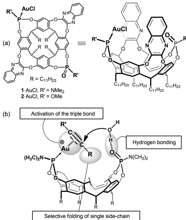
Figure 1. (a) Mono-AuCl cavitands **1**·AuCl and **2**·AuCl, and (b) working hypothesis of three points: (1) coordination of Au<sup>+</sup> toward an alkyne triple bond, (2) hydrogen bonding between P=O and H<sub>2</sub>O, and (3) selective folding of single side chain (the two quinoxaline walls are omitted for ease of viewing).
